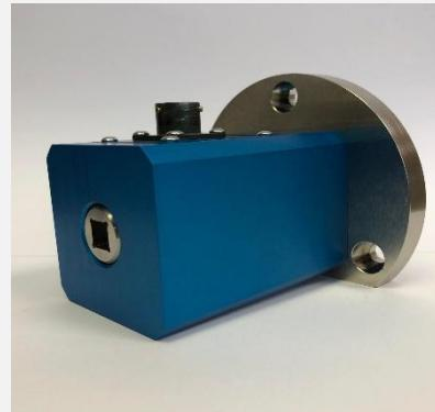
The IITT is attached to the ITMB using a pattern of either 2 M4 Bolts (ITT-1018) or 4 M5 Bolts (IITT-1012-1016 &1070). These are bolted into the reaction end of the transducer housing.
