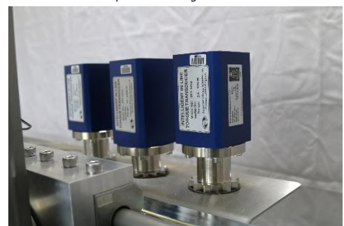
AWS Intelligent Inline Torque Transducers with spline drive adapters for fitting into the UTWCM
