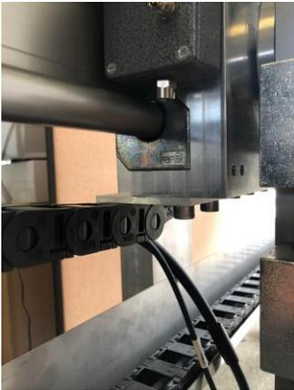
20. Connect the grey motor cable to the stepper motor.
