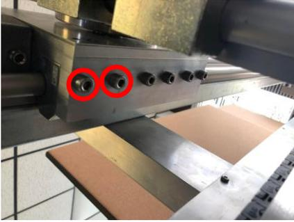
19. Attach the Cable chain plate where the M8 bolts were removed using the same bolts.
