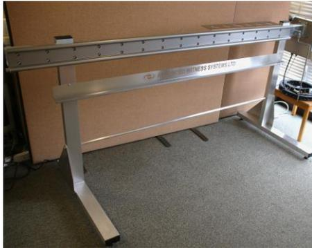
8. Prop the machine on a block of wood or similar (one stand at a time) to gain access to the M8 levelling feet mounts beneath the horizontal box sections.
