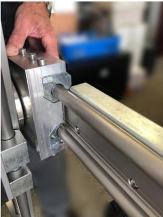
16. Attach the M12 bolt to the rear of the main track.
