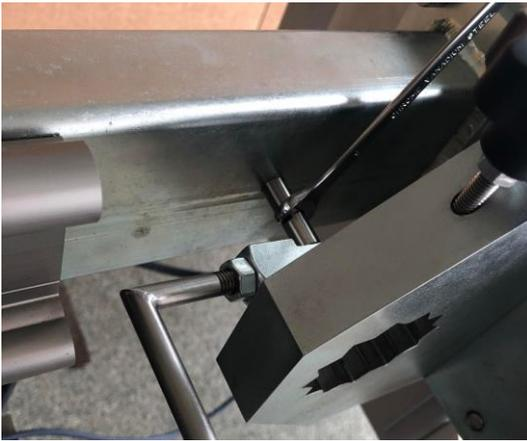
15. Slide the main carriage onto the track, ensuring that the connector box for the Travel Limit Sensors is facing away from the Control Box end of the machine.
