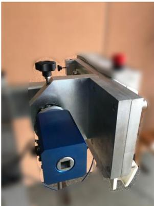
2. Tighten the Transducer Retaining Screw to hold the transducer in place.
