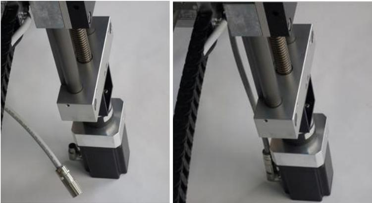
21. Connect the sensor cable from the control box to the lid of the Travel Limit Sensor box on the rear of the main carriage.
