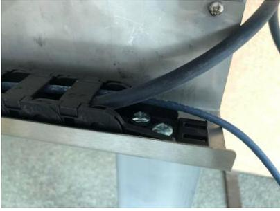
14. Attach the reaction rod assembly in the hole beneath the transducer cassette using an 8 or 10mm spanner.
