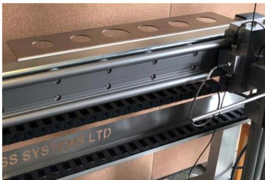
12. Attach the Control Box to the end of the machine using the four long M4 bolts (this may already be attached on the machine for shipping).
