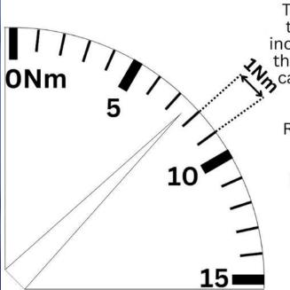
The pointer tip is less than 1/5 of the scale increment, meaning that the resolution available can be 1/5 of the scale increment value.
