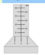
Smallest increment is on secondary scale
