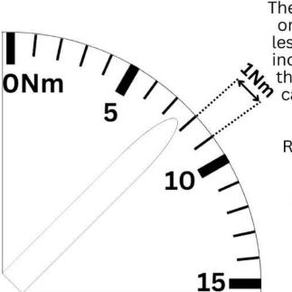
The pointer tip is equal to or greater than 1/5, but less than 1/2 of the scale increment, meaning that the resolution available can be 1/2 of the scale increment value.
