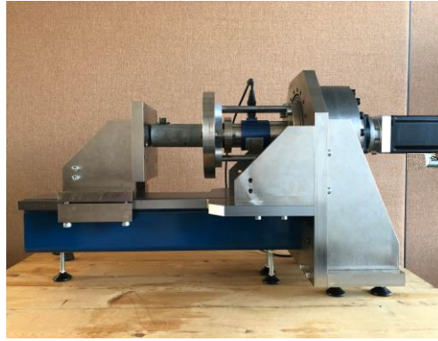
Bench mounted machine with Torque Transducer Sliding Carriage and 2kNm Master Transducer, alongside the control box.
