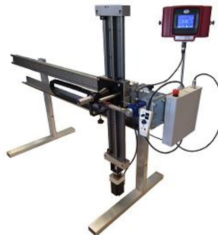
UTWCM with 60N-m Torque Wrench
