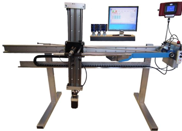
Photo above shows a UTWCM with AWS Intelligent Inline Torque Transducers, Professional Transducer Display, and Laptop/Computer running ADMS Kepler 4 Software for Calibration & Conformity to ISO 6789:2017 Parts 1 and 2.
